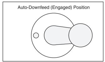
**Figure 37.** Downfeed selector in auto-downfeed (engaged) position.
